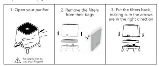
Note: if you're using a carbon filter, make sure you insert it in the right order: Carbon filter (bottom) → HEPA filter (top)
